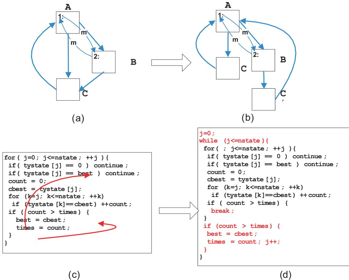
Figure 5.12: Example of dependence isolation: (a) mechanics of transformation for an abstract loop, (b) example loop from yacc.
