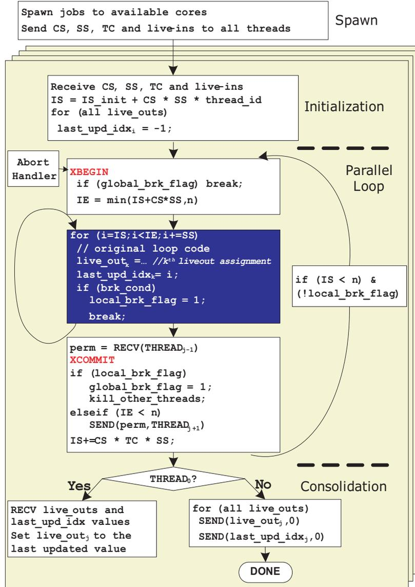
Figure 5.7: Detailed code generation framework for speculative loop parallelization. Transaction scope is marked by XBEGIN and XCOMMIT. (CS: chunk size, IS: iteration start, IE: iteration end, SS: step size, TC: thread count)
