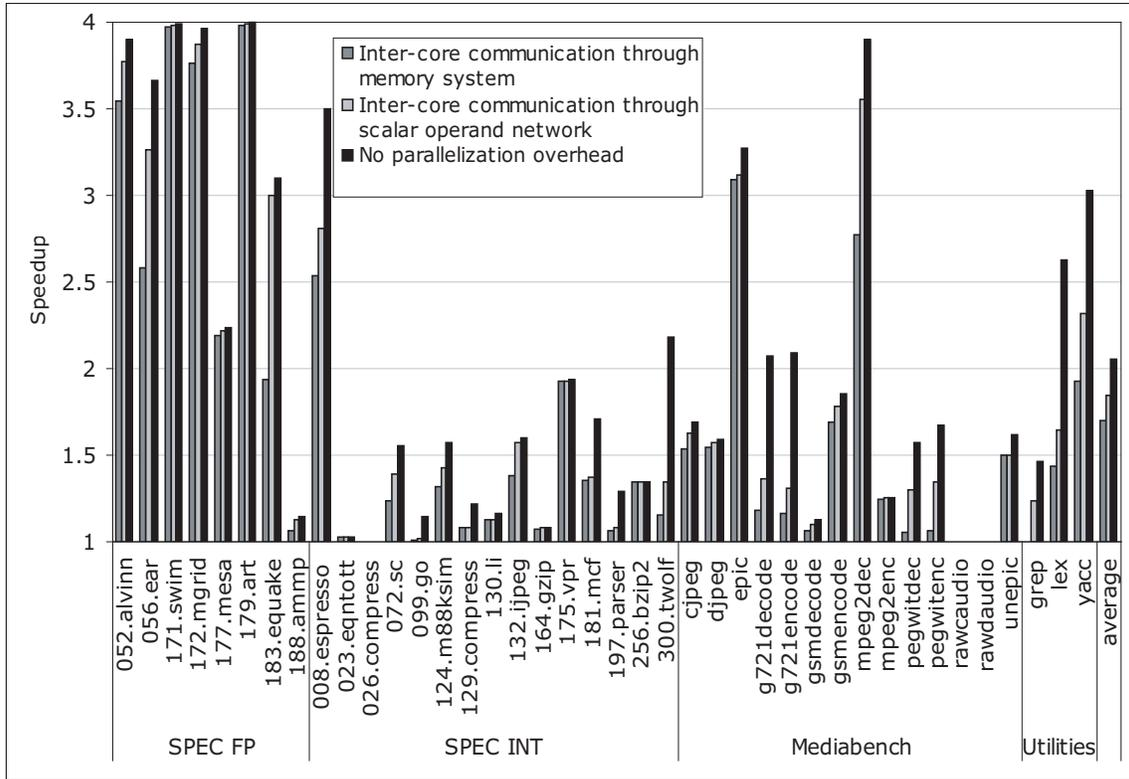
Figure 6.12: The first two bars show the effect of inter-core communication through memory systems versus scalar operand network. The last bar shows the speedup without any parallelization overhead.
