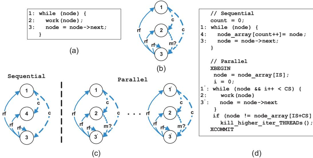
Figure 5.8: Speculative loop fission (a) Original loop (b) Original data flow graph (c) Data flow graph after fission (d) Loop after fission - (rf: register flow dependence, c: control dependence, m?: unlikely cross-iteration memory dependence)
