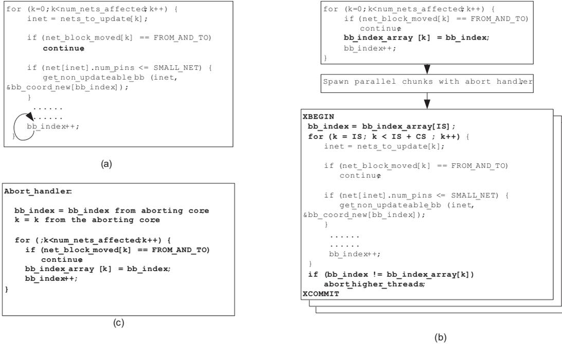
Figure 5.9: Example of speculative loop fission from 175.vpr: (a) original loop (b) loop after fission (c) abort handler.
