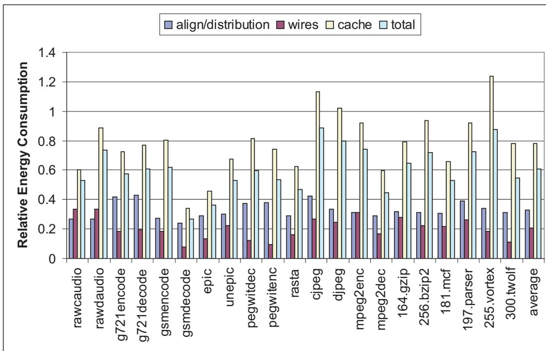
Figure 6.4: Relative energy consumption for the instruction fetch subsystem of a 4-cluster DVLIW processor.
