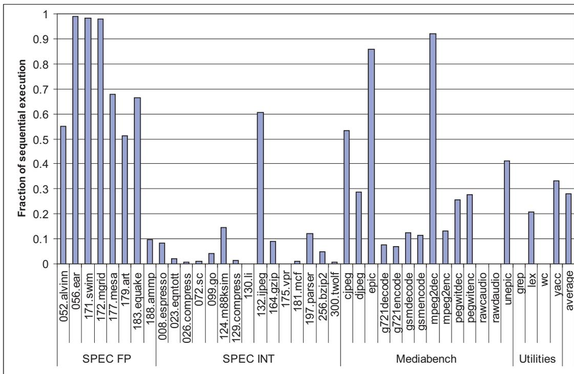
Figure 5.4: Fraction of sequential execution covered by DOALL loops identified through profiling analysis.
