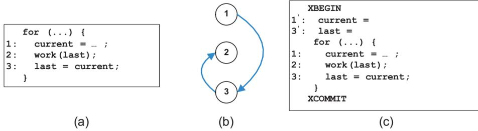
Figure 5.10: Example of speculative prematerialization: (a) original loop, (b) dataflow graph, and (c) loop after transformation.
