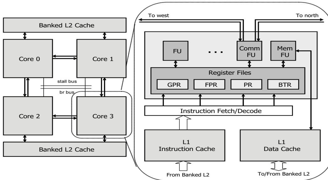
Figure 3.1: Overview of multicore architecture for ILP execution. Four core example is shown.
