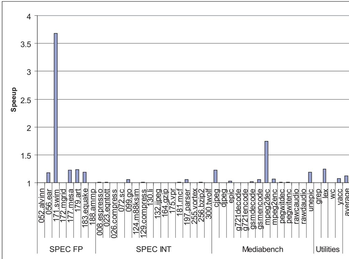
Figure 5.2: Potential speedup for idealized CMP using DOALL loops identified through compiler analysis.
