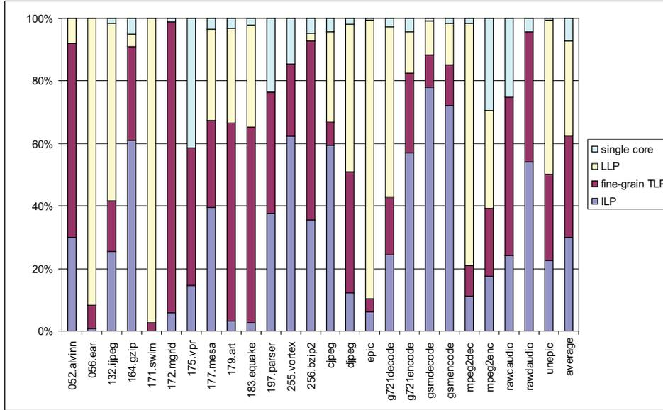
Figure 2.5: Breakdown of exploitable parallelism for a 4-core system.
