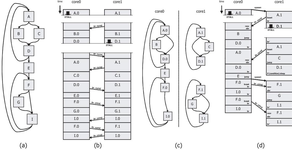
Figure 3.8: Code execution under different modes. (a) Control flow graph of a code segment. (b) Execution of the code segment under coupled mode. (c) Control flow graph of fine-grain threads extracted for decoupled mode. (d) Execution of the code segment under decoupled mode.
