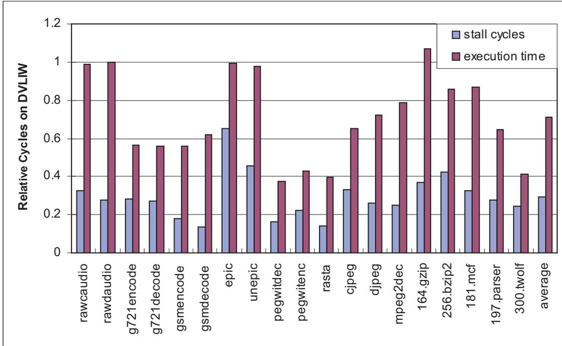
Figure 6.7: Comparison of the relative stall cycles and execution time on a 4-cluster DVLIW with a VLIW having a distributed I-cache and a shared PC.
