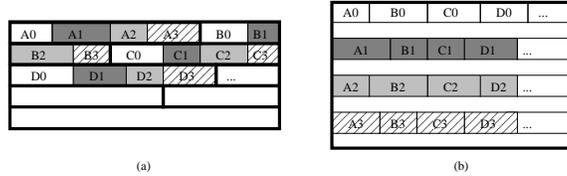
Figure 3.2: (a) Code layout on a conventional 4-cluster VLIW architecture. Rectangle A0 represents operations in MultiOp A to be executed by cluster 0. (b) Code layout on the proposed multicore architecture. Bold lines represent MultiOp boundaries in (a).
