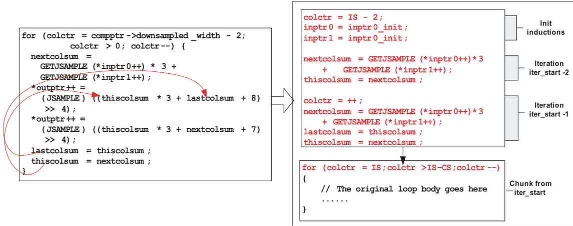
Figure 5.11: Example of speculative prematerialization from djpeg.
