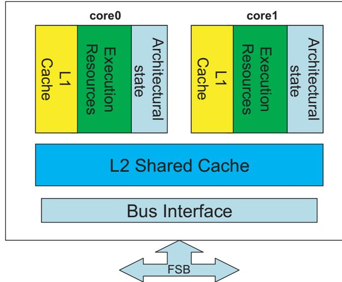
Figure 2.1: A 2 core CMP architecture
