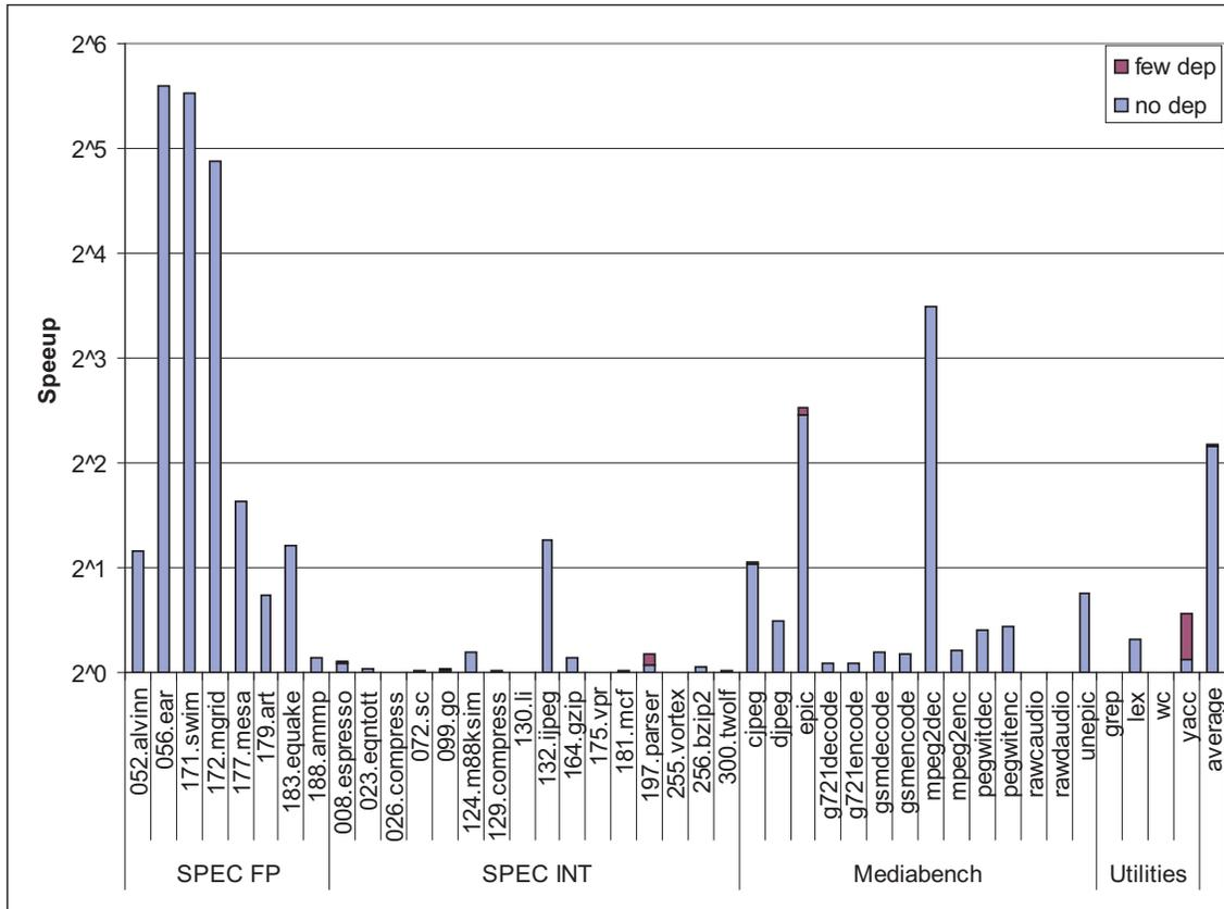
Figure 5.5: Potential speedup for idealized CMP using DOALL loops identified through profiling analysis.
