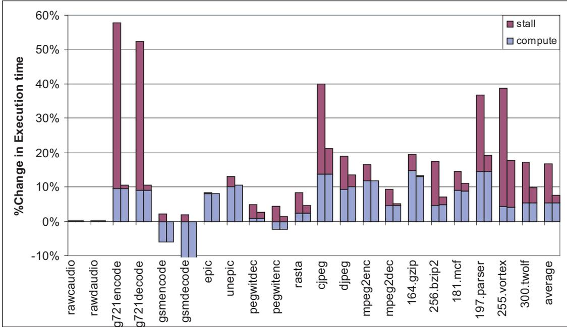
Figure 6.2: Relative execution time on a 4-cluster DVLIW processor with total I-cache sizes of 16K and 32K.
