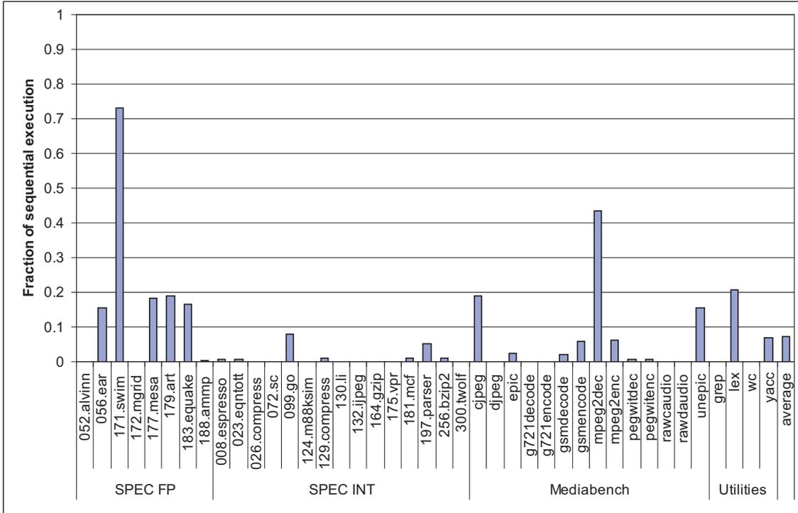
Figure 5.1: Fraction of sequential execution covered by DOALL loops identified through compiler analysis.
