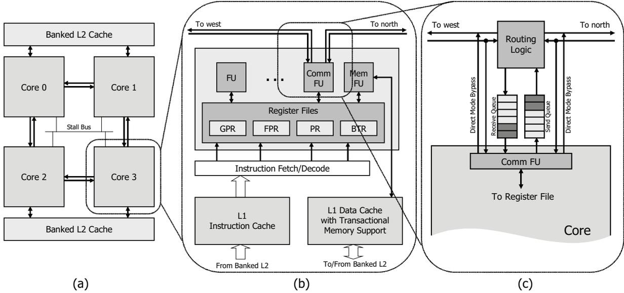
Figure 3.6: Block diagram of the Voltron architecture: (a) 4-core system connected in a mesh topology, (b) Datapath for a single core, and (c) Details of the inter-core communication unit.
