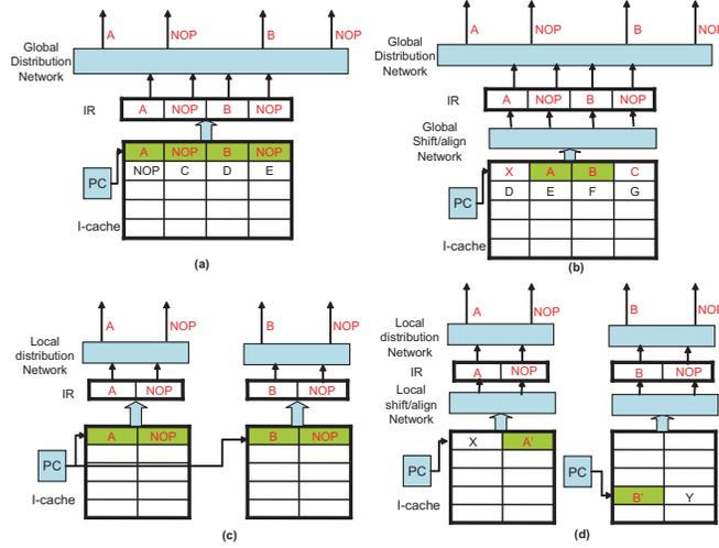
Figure 3.5: Instruction memory organizations: (a) Centralized instruction cache, uncompressed encoding; (b) Centralized instruction cache, compressed encoding; (c) Distributed I-cache, centralized PC, uncompressed encoding; (d) Distributed I-cache, distributed PC, compressed encoding.
