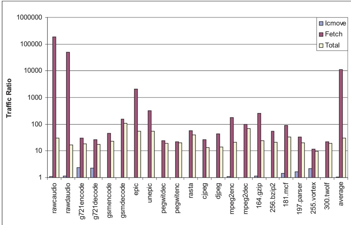
Figure 6.3: Reduction in dynamic global communication signals of a 4-cluster DVLIW processor.
