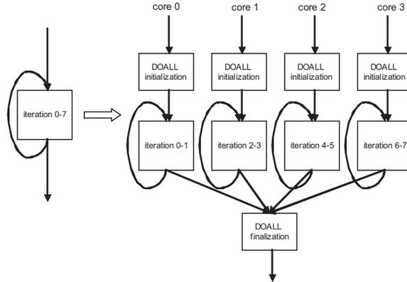
Figure 2.4: Example of Loop Level Parallelism
