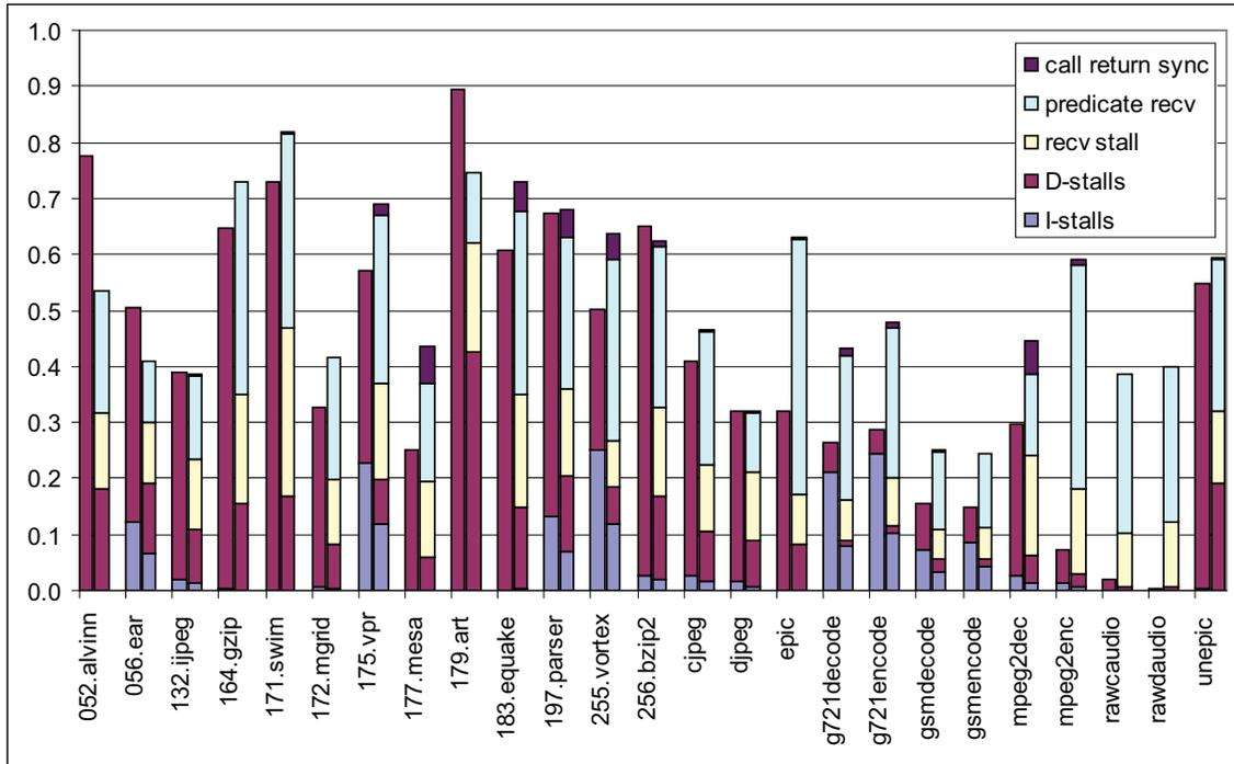
Figure 6.9: Breakdown of synchronization stalls by type on a 4-core system. Each benchmark has two bars: the left bar is for decoupled mode and the right for coupled mode.
