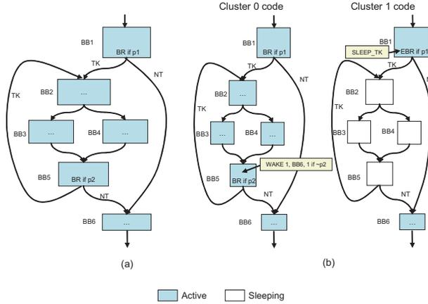
Figure 3.4: Sleep mode example: (a) Original control flow graph, (b) control flow graphs for a 2-core architecture where core one is in sleep mode for blocks two through five. Sleep mode is entered via the SLEEP\_TK operation in BB1 on Cluster 1 and exited via the WAKE operation in BB5 on Cluster 0.
