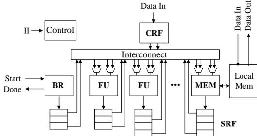
Figure 2: Hardware schema for loop accelerator.
